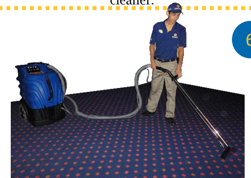
With the equipment for washing carpets and seats, inject detergent forming a line the width of the tube (handle) of the equipment and go over it three times extracting detergent on the same line. Repeat process from 5 to 7 times.
