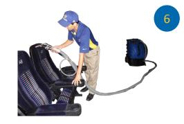
With the equipment for washing carpets and seats, inject detergent forming a line the width of the tube (handle) of the equipment and go over it three times sucking on the same line. Repeat process from 5 to 7 times.
