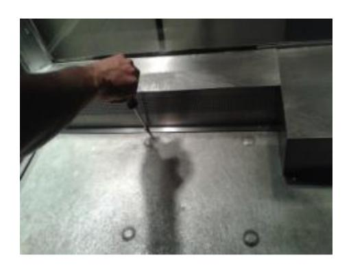
Step 4- Unscrew the thermostat at the base. There are two screws at the extremes of the protective case.
