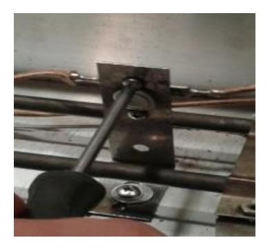
Step 5- The thermostat has two power terminals that are necessary to remove before removing the thermostat.
