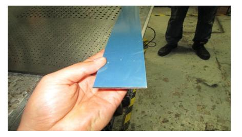
Utilize a carbon steel sheet with mirror finish of 22 gauge.
